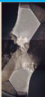
110穴加工後 After 110 holes
