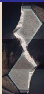
180穴加工後 After 180 holes
